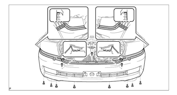
f. w/ Headlight Cleaner System: Disconnect the headlight cleaner hose and remove the bumper cover.
