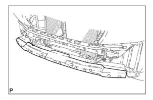
8. REMOVE FRONT BUMPER REINFORCEMENT SUB-ASSEMBLY
