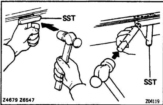
**19. REMOVE OIL PAN BAFFLE PLATE**
