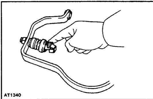
(b) Install the cross shaft to the body.
