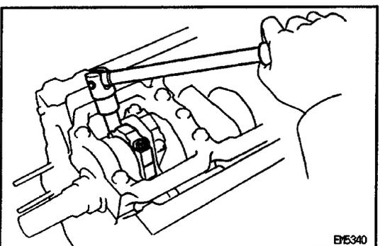
(b) Remove the connecting rod cap nuts.
