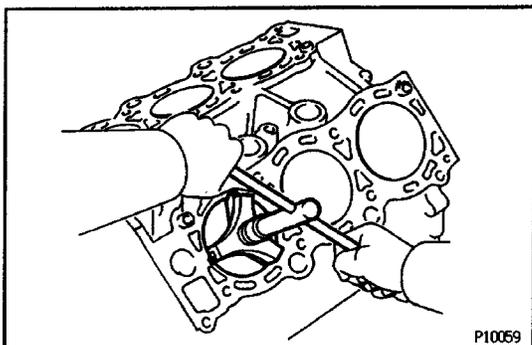
**4. REMOVE PISTON AND CONNECTING ROD ASSEMBLIES**
