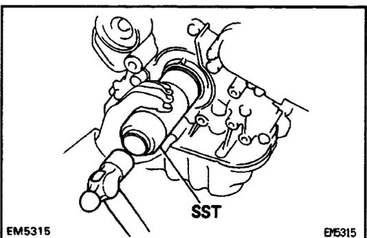
(c) Apply NIP grease to a new oil seal lip.
