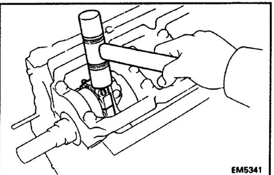
(c) Using a plastic-faced hammer, lightly tap the connecting rod bolts and lift off the connecting rod cap.
