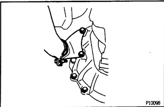
(c) Install the pipe bracket to the transmission with the 2 bolts.
