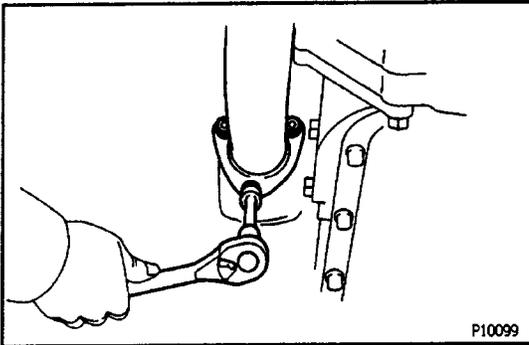
**16. INSTALL FRONT EXHAUST PIPE**
