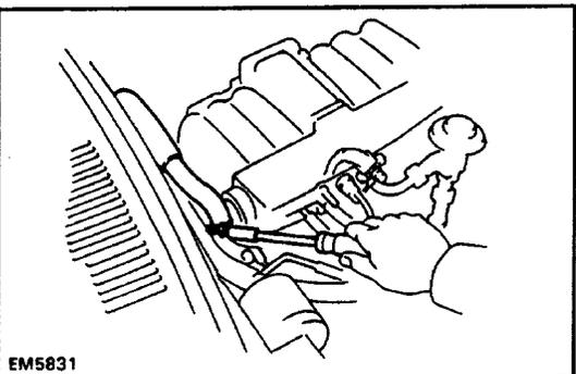
**19. CONNECT HEATER HOSES****20. CONNECT FUEL INLET AND OUTLET HOSES**
