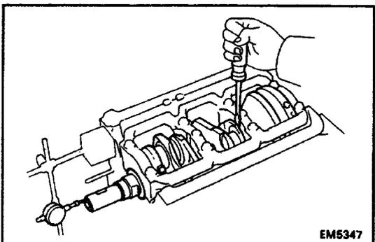
**5. CHECK CRANKSHAFT THRUST CLEARANCE**
