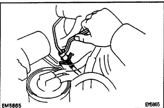
**17. M/T only:****CONNECT CLUTCH RELEASE CYLINDER HOSE****18. INSTALL A/C COMPRESSOR**
