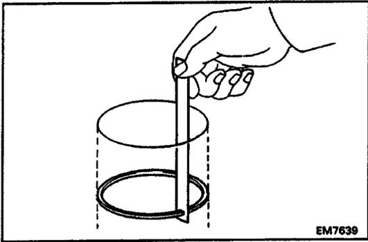
(c) Using a feeler gauge, measure the ring end gap.
