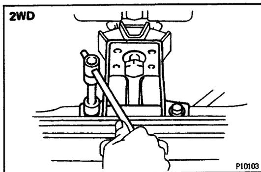
(b) Raise the transmission slightly by raising the engine with a jack.
