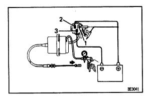
(d) Disconnect terminal 1 or 2 and check that the control cable returns to its original position and the vacuum returns to 0 kPa (0 mmHg, 0 in.Hg).
