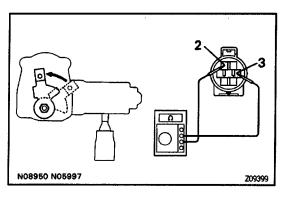
(b) When the arm is moving from the closed to open position, check that resistance between terminal 2 and 3 increases from approx. 0.5 to 1.8 k $\Omega$ . If operation is not as specified, replace the motor.
