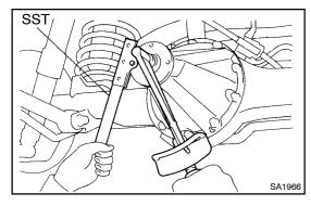
(c) Using SST to hold the flange, install the nut.
