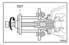
(c) Using SST, remove the companion flange. SST 09950-30010 (09951-03010, 09953-03010, 09954-03010, 09955-03030, 09956-03040)
