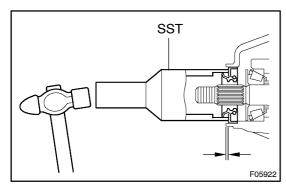
(c) Using SST and a hammer, install a new oil seal. SST 09214-76011
