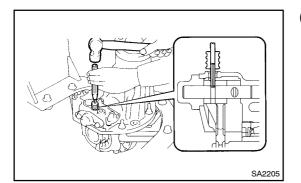
(h) Using a pin punch and hummer, install the slotted spring pin to the shift fork.
