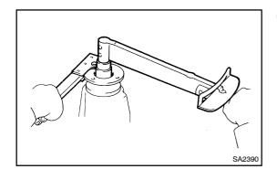
Using SST to hold the flange, tighten the nut. SST 09330-00021
