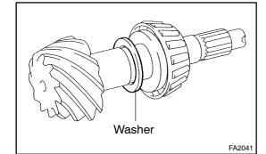
If the teeth are not contacting properly, use the following chart to select a proper washer for correction.
