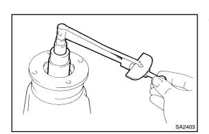
Using a torque wrench, measure the preload.
