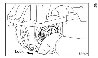
) Shift the fork deeply and keep the differential lock condition.
