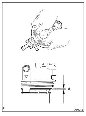
(d) Push the cap into the case by hand.
