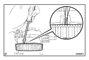
(g) Fully loosen the fastener nut by hand.
