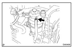
Connect the hose to the filter outlet side and install the clip (g) as shown in the illustration.
