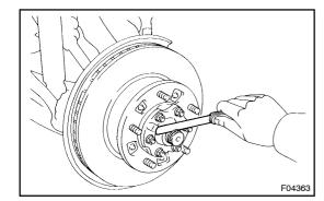
(d) Pull out the drive shaft outside the vehicle and select the snap ring which ensures the clearance between the tip of the flange and the snap ring is less than 0.2 mm (0.008 in.).
