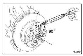
(d) Using a spring tension gauge, check the preload. **Preload (at starting):**
