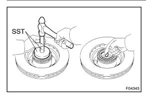
(b) Using SST and a hammer, install a new oil seal into the axle hub.
