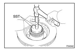
(b) Using SST and a hammer, carefully install a new inside bearing outer race.
