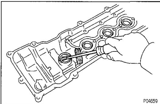
**16. IF NECESSARY, REPLACE SPARK PLUG TUBE GASKETS**
