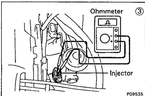
③ Check resistance of each injector. STD resistance: Approx. 13.8 Ω
