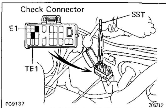
3. Using SST, connect terminals TE1 and E1 of the check connector.
