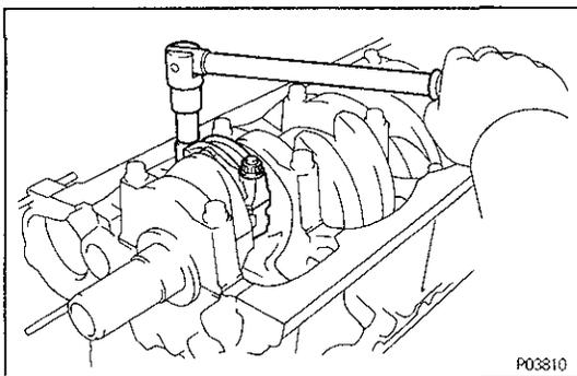
(c) Using a plastic-faced hammer, lightly tap the connecting rod bolts and lift off the connecting rod cap. **HINT:** Keep the lower bearing inserted with the connecting rod cap.
