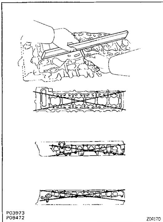
**3. INSPECT CYLINDER HEAD****A. Inspect for flatness**
