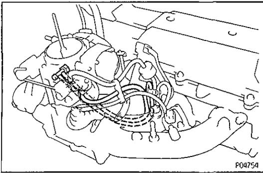
**22. CONNECT TWO VACUUM HOSES TO BVS**
