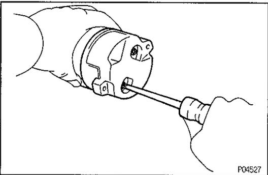
**3. INSERT STEEL BALL INTO CLUTCH SHAFT HOLE**
