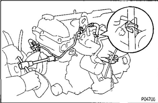
**23. INSTALL NO.2 WATER BY-PASS PIPE AND HOSES**
