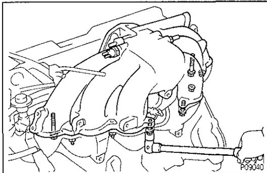
(b) Remove the four bolts, six nuts, air intake chamber and two gaskets.
