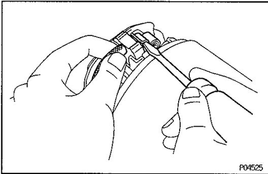
(c) Place a new O-ring in position on the field frame.
