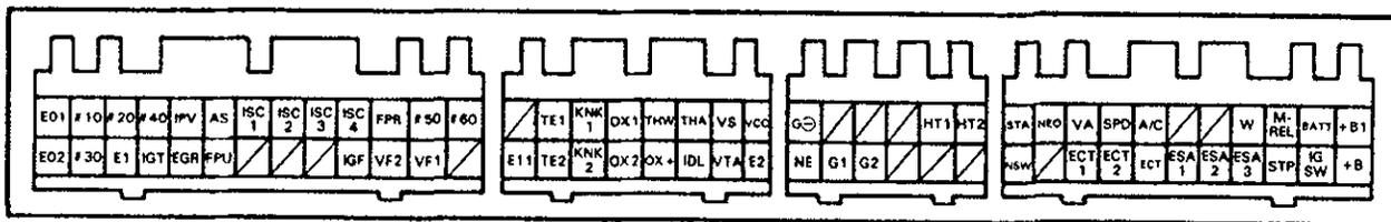
ECU Wiring Connectors Voltage (For A/T)
