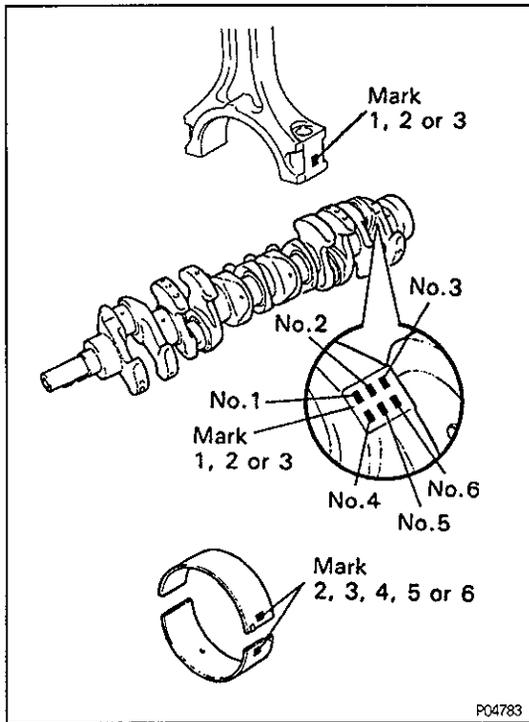
**HINT:** If using a standard bearing, replace with one having the same number. If the number of the bearing cannot be determined, select the correct bearing by adding together the numbers imprinted on the connecting rod and crankshaft, then selecting the bearing with the same number as the total. There are five sizes of standard bearings, marked "2", "3", "4", "5" and "6" accordingly.
