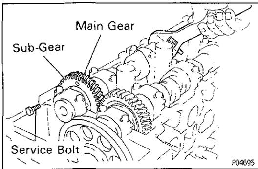
**A. Remove exhaust camshaft**
