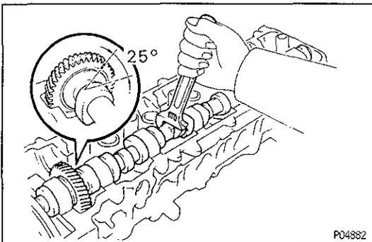
**B. Remove intake camshaft**
