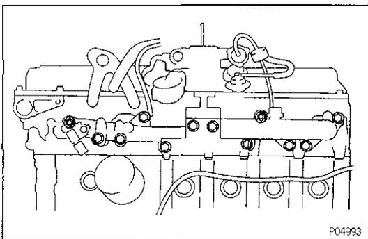
**14. REMOVE INTAKE MANIFOLD WITH CARBURETOR**
