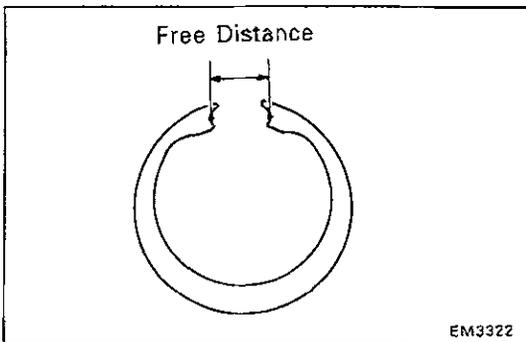
**E. Inspect camshaft gear spring**
