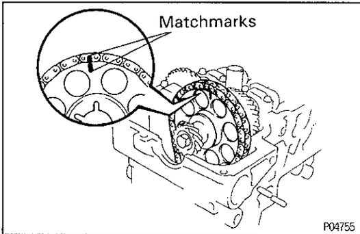
**24. REMOVE CAMSHAFT TIMING GEAR**
