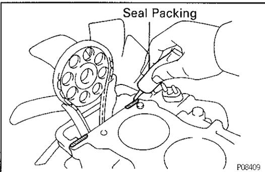
**5. INSTALL CYLINDER HEAD****A. Place cylinder head on cylinder block**
