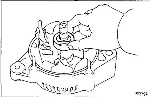
(c) Remove the thrust washer.
