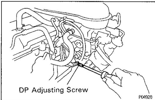
If the DP setting speed is not as specified, adjust the setting speed by turning the DP adjusting screw.
