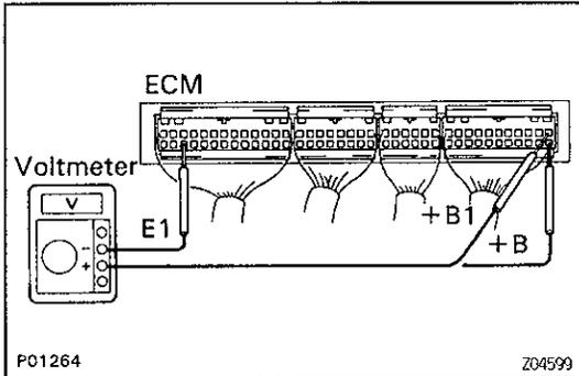
(b) Measure the voltage between each terminal of the wiring connectors.
