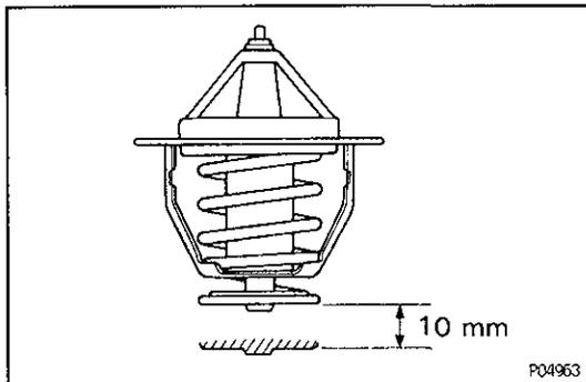
(c) Check the valve lift.
