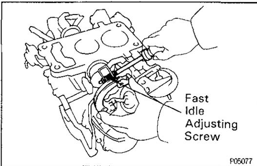
(d) Adjust by turning the fast idle adjusting screw.
