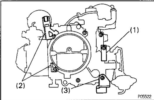
(b) Place the air horn in the carburetor body.
