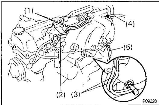
**12. REMOVE AIR INTAKE CHAMBER**
