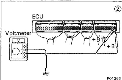
② Check that there is voltage between ECU terminal +B (+B1) and body ground. (IG SW ON)
