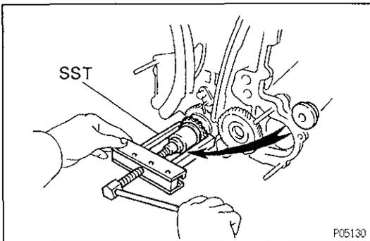
HINT: If necessary, remove the gear with SST.
