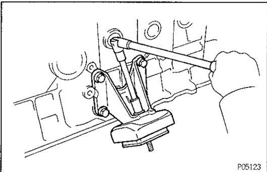
**10. REMOVE LH ENGINE MOUNTING BRACKET**
