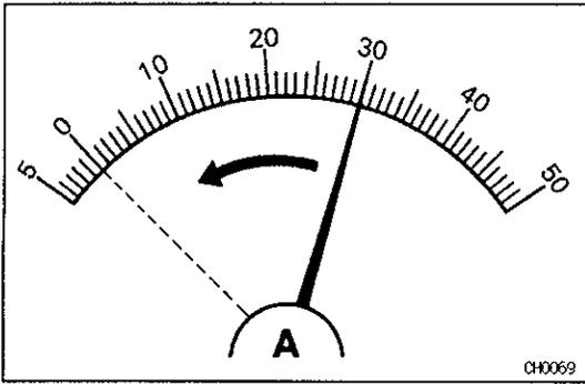
If the ammeter reading is less than standard amperage, repair the alternator.
