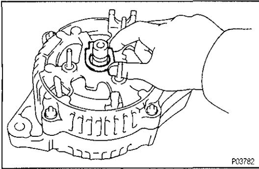
(c) Remove the seal plate.
