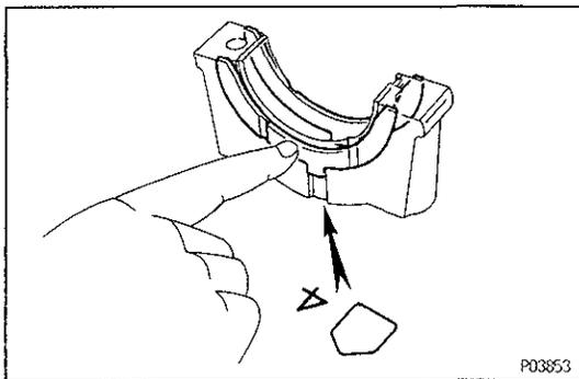
**6. INSTALL MAIN BEARING CAPS AND LOWER THRUST WASHERS**
