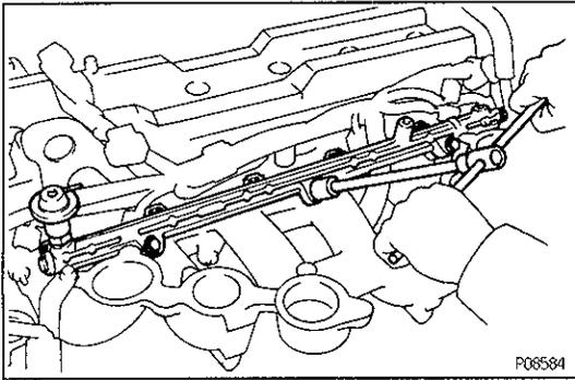
**17. REMOVE DELIVERY PIPE AND INJECTORS**
