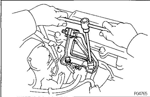
**12. REMOVE ACCELERATOR CABLE BRACKET**
