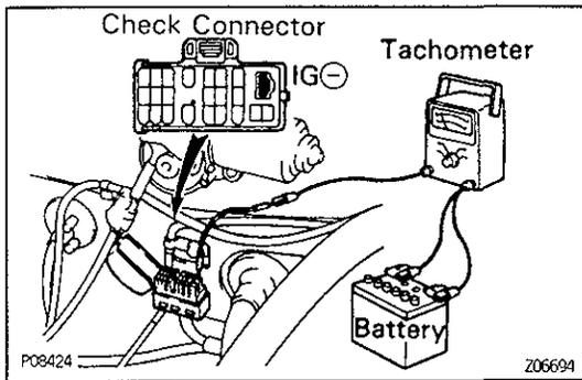
**8. CONNECT TACHOMETER AND TIMING LIGHT**
