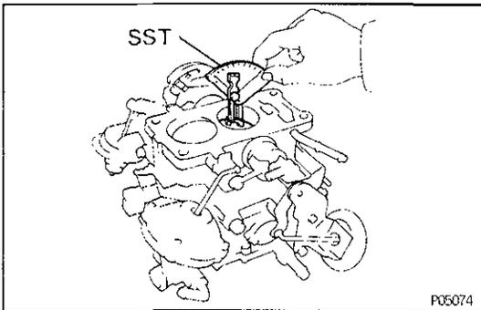
(c) Check the primary throttle valve angle.
