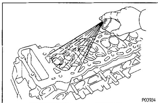
**B. Inspect for cracks**
