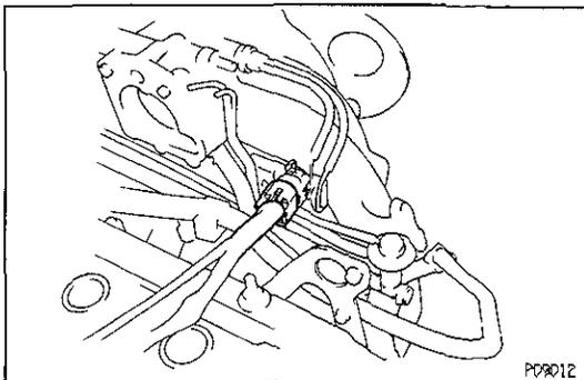
**34. CONNECT CONNECTOR FOR EMISSION CONTROL VALVE SET ASSEMBLY**
