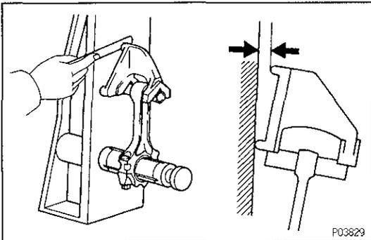
**3. INSPECT CONNECTING ROD****A. Inspect connecting rod alignment**
