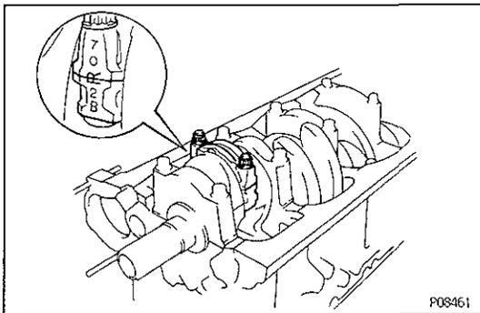
(b) Remove the connecting rod cap nuts.
