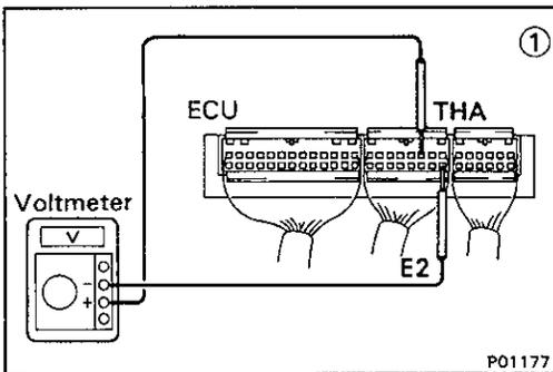
① There is no voltage between ECU terminals THA and E2. (IG SW ON)
