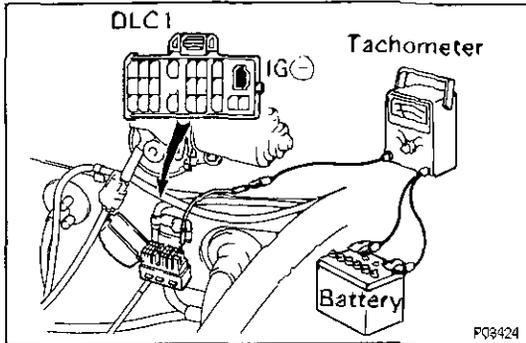
Using SST, connect terminals TE1 and E1 of the check connector
