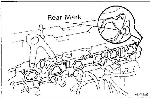
**18. INSTALL INTAKE MANIFOLD WITH CARBURETOR**
