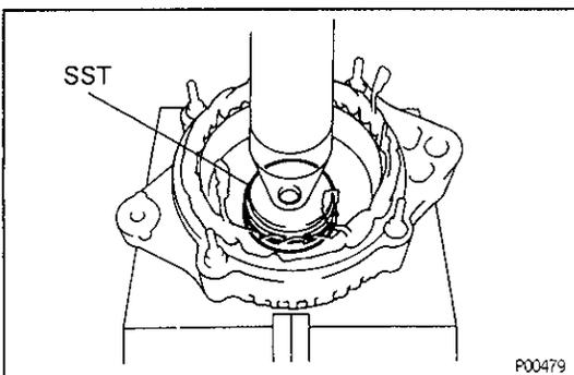
(c) Using SST and a press, press in a new bearing.
