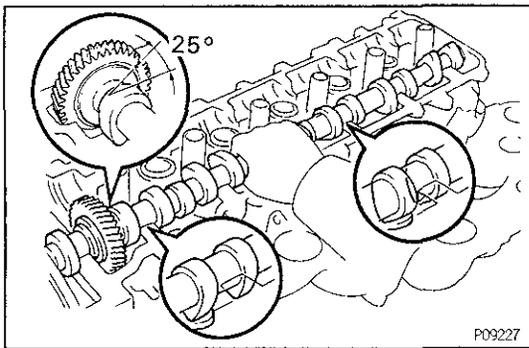
**A. Install intake camshaft**
