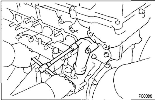
**25. REMOVE WATER BY-PASS OUTLET AND PIPE**
