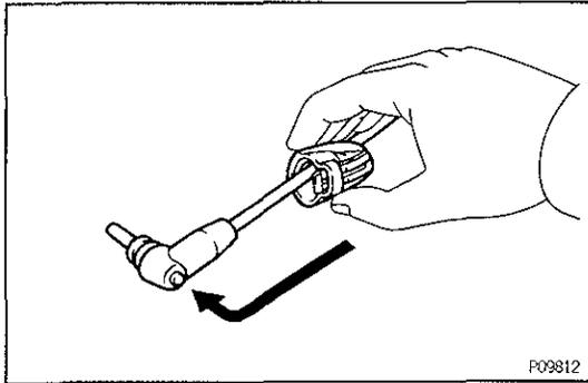
**5. RECONNECT HIGH – TENSION CORDS TO DISTRIBUTOR CAP AND IGNITION COIL**
