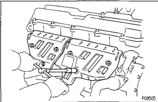
**22. REMOVE NO.1 AND NO.2 EXHAUST MANIFOLDS**
