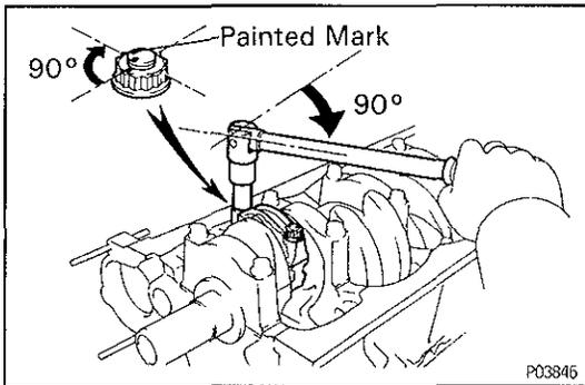
(d) Retighten the connecting rod cap nuts 90° as shown.
