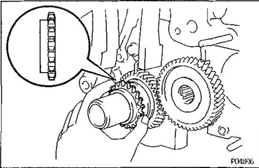
HINT: If necessary, install the gear with SST.
