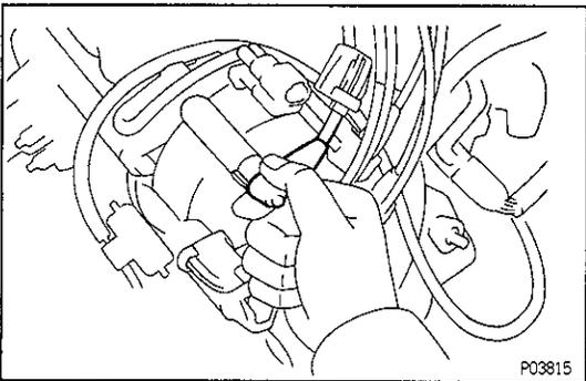
**6. RECONNECT HIGH–TENSION CORDS TO DISTRIBUTOR CAP AND IGNITION COIL**
