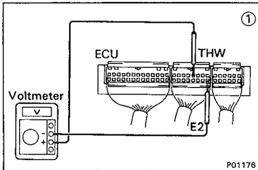
① There is no voltage between ECU terminals THW and E2. (IG SW ON)
