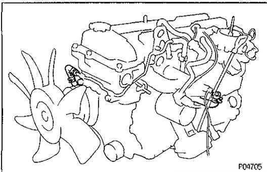
**9. REMOVE NO. 2 WATER BY – PASS PIPE WITH HOSES**
