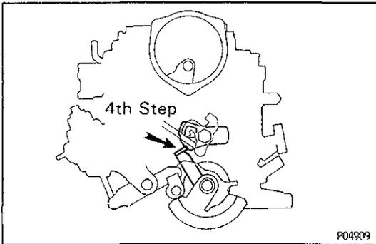
(b) Position the fast idle lever onto the 4th step as shown.
