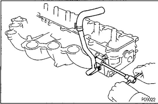
**3. INSTALL HEATER INLET PIPE AND HOSE**
