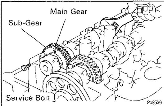
**A. Remove exhaust camshaft**
