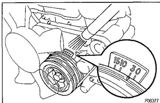
(b) Using a timing light, check the ignition timing.
