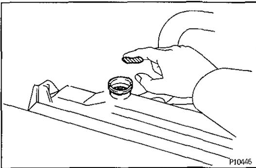
(b) There should not be any excessive deposits of rust or scales around the radiator cap or radiator filler hole, and the coolant should be free from oil.
