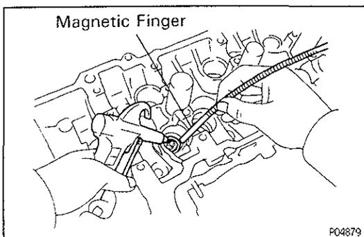
(d) Using compressed air and magnetic finger, remove the spring seat by blowing air.
