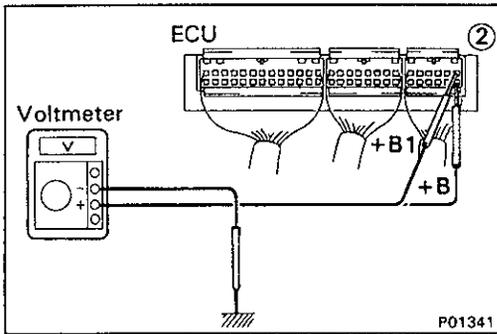
Check wiring between ECU terminal E1 and body ground.
