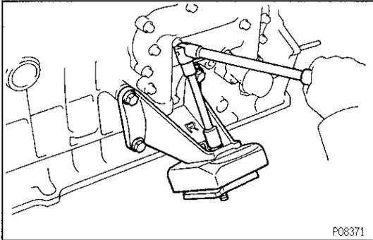
**9. REMOVE RH ENGINE MOUNTING BRACKET**
