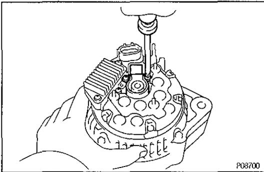
(b) Remove the two screws and brush holder.
