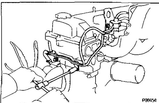
**35. INSTALL NO.2 WATER BY-PASS PIPE AND HOSES**
