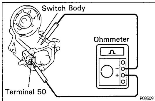
2. **PERFORM HOLD-IN COIL OPEN CIRCUIT TEST**
