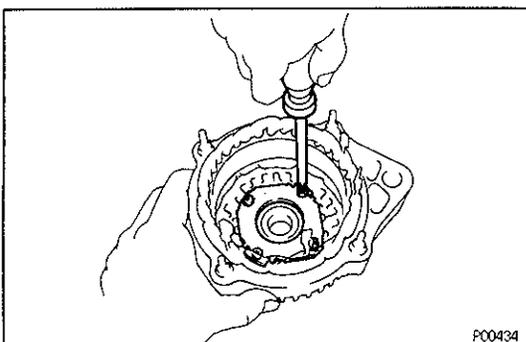
(d) Install the bearing retainer with the four screws.
