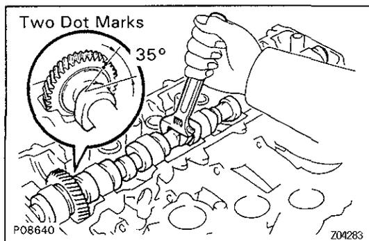
**B. Install exhaust camshaft**
