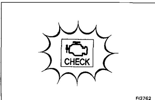
4. Read the diagnostic code as indicated by the number of flashes of the "CHECK" engine warning light.
