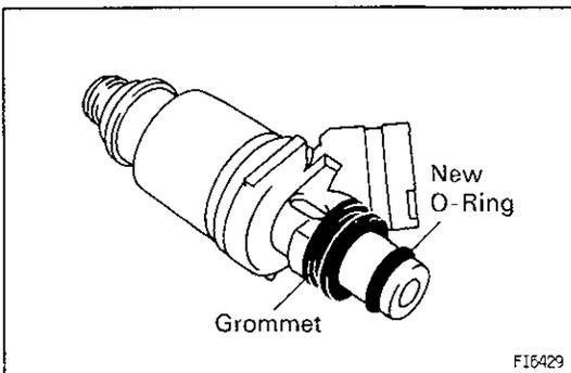
**25. INSTALL INJECTORS AND DELIVERY PIPE**
