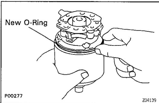
(d) Install a new O-ring to the the end cover screw.
