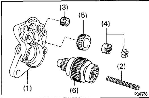
(b) Remove the following parts from the magnetic switch assembly:
