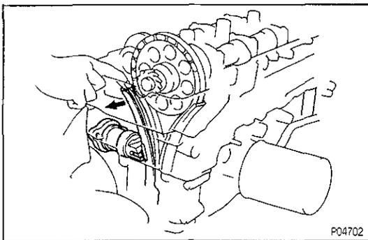
**HINT:** If the plunger does not spring out, press the slipper into the chain tensioner with a screwdriver or your finger so that the hook is released and the plunger springs out.
