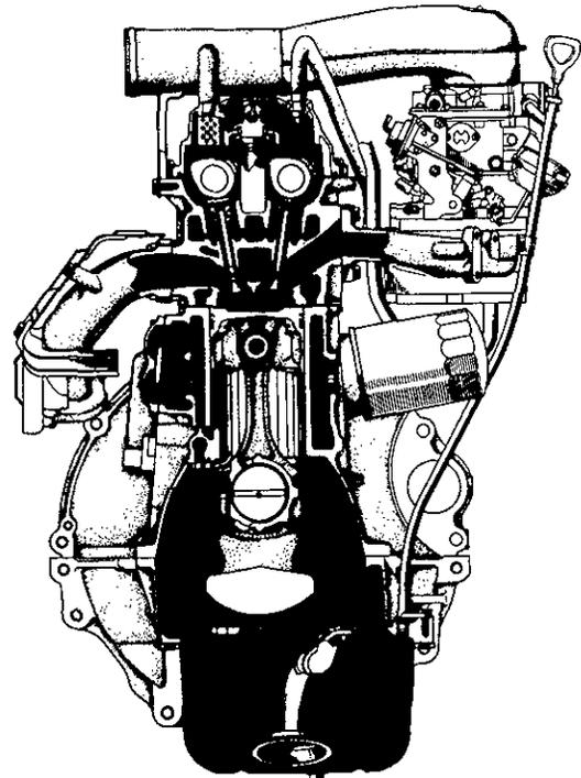
The 1FZ–FE and 1FZ–F engines are an in–line, 6–cylinder engine with the cylinders numbered 1–2–3–4–5–6 from front. The crankshaft is supported by 7 bearings inside the crankcase. These bearings are made of aluminum alloy.
