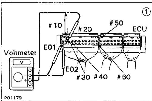
① There is no voltage between ECU terminals # 10 ~ # 60 and E01 and/or E02. (IG SW ON)
