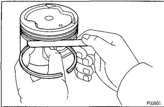
**B. Inspect piston ring groove clearance**
