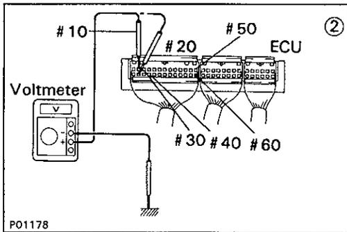
② Check that there is voltage between ECU terminal # 10 ~ # 60 and body ground.
