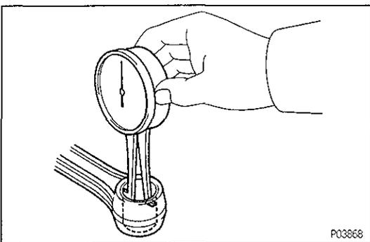
**B. Inspect piston pin oil clearance**
