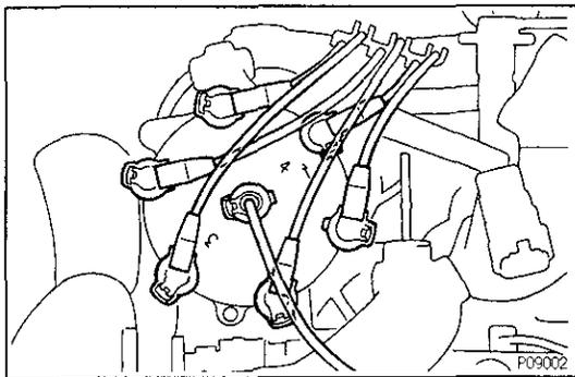
**HINT:** Connect the high–tension cords to the distributor cap as shown in the illustration.
