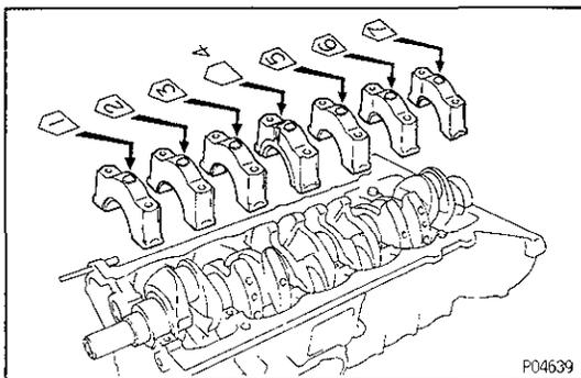
(b) Install the seven main bearing caps in their proper locations.
