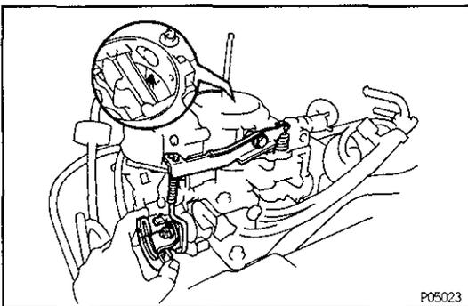
**14. INSTALL AIR INTAKE CONNECTOR****15. CHECK AND ADJUST IDLE SPEED AND IDLE MIXTURE****16. CHECK AND ADJUST FAST IDLE SPEED****17. CHECK AND ADJUST DASH POT (DP) SETTING SPEED****18. CHECK AND ADJUST THROTTLE POSITIONER (TP) SETTING SPEED**
