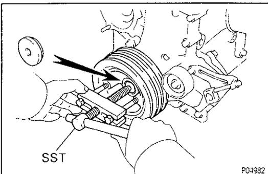
**HINT:** If necessary, remove the pulley with SST.
