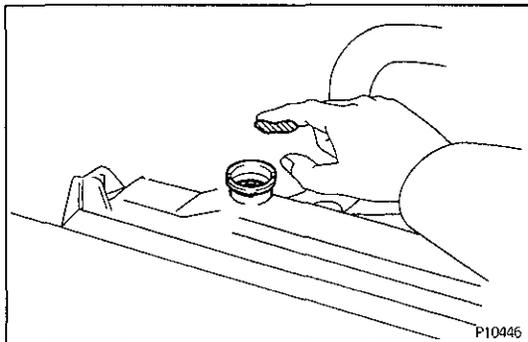
(b) There should not be any excessive deposits of rust or scales around the radiator cap or radiator filler hole, and the coolant should be free from oil. If excessively dirty, replace the coolant.
