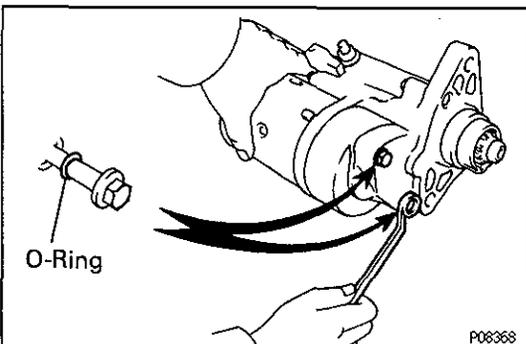
(b) Remove the two through bolts and O-rings.
