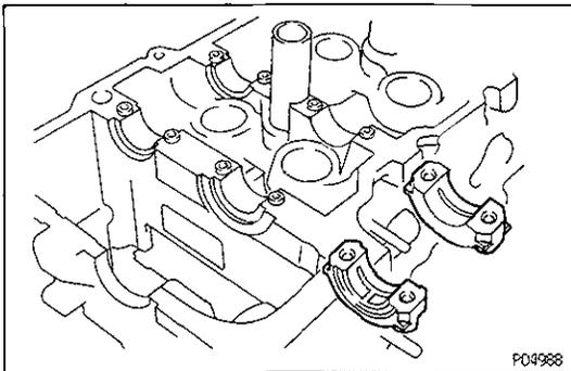
**D. Inspect camshaft bearings**
