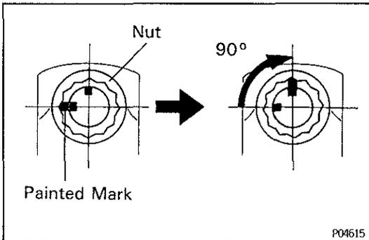
(e) Check that the painted mark on the nut is at 90° angle in relation to the mark on the bolt.
