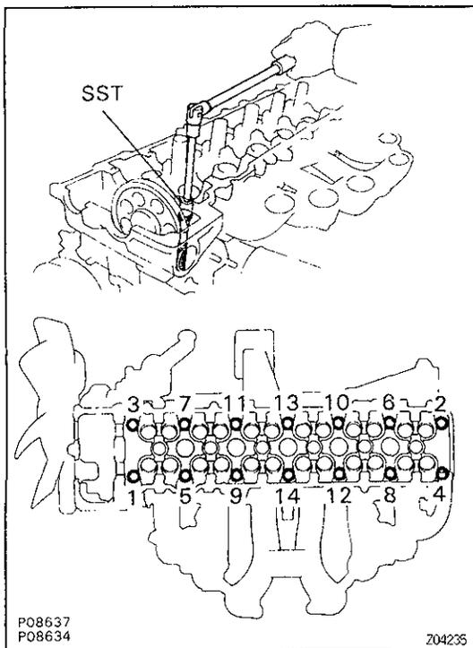
(b) Using SST, uniformly loosen and remove the 14 cylinder head bolts in several passes, in the sequence shown.
