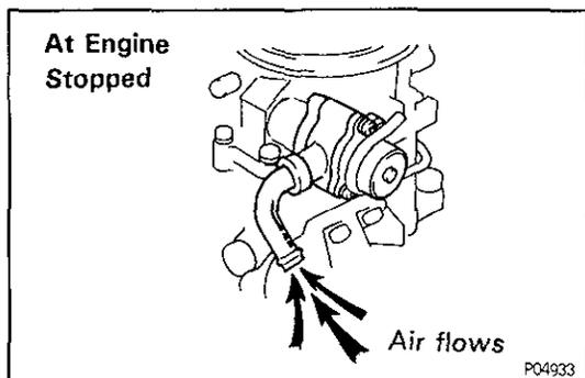
**8. INSPECT OUTER VENT CONTROL VALVE (OVCV) OPERATION**
