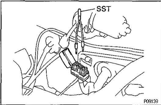
(e) Remove SST from the check connector.
