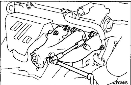
(b) Remove the six nuts, exhaust manifold and gasket.
