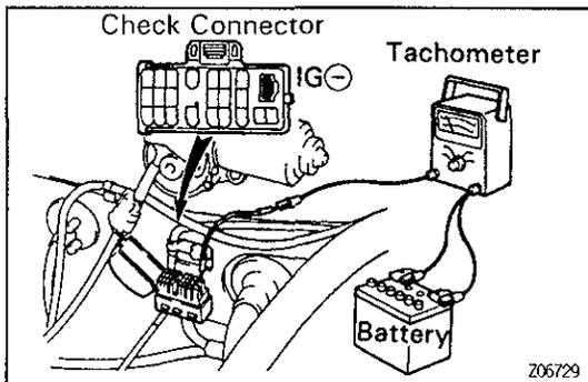
2. With a tachometer connected to the system, connect the test probe of the tachometer to the IG $\ominus$  of the check connector.
