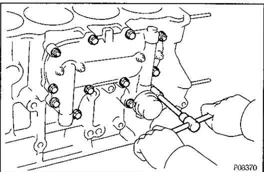
**11. REMOVE OIL COOLER COVER AND OIL COOLER**
