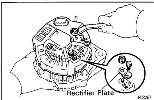
(b) Remove the three nuts, screw, rectifier plate and end cover.
