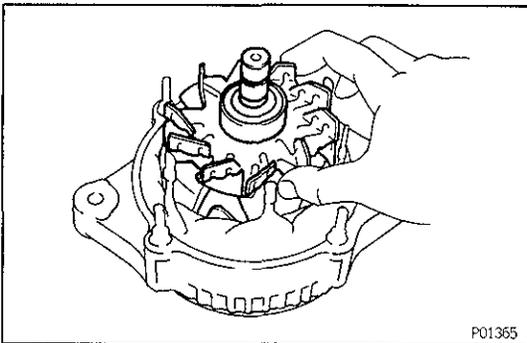
**7. REMOVE ROTOR FROM DRIVE END FRAME**
