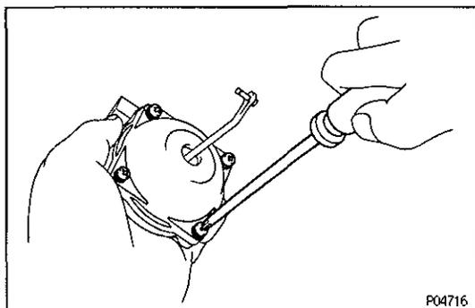
(c) If necessary, remove the four screws and disassembly the throttle valve diaphragm.
