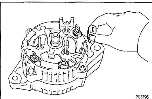
(b) Remove the four rubber insulators.
