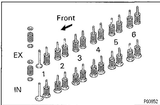
**HINT:** Arrange the valves, valve springs, spring seats and spring retainers in correct order.
