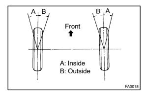
(b) Turn the steering wheel fully, and measure the turning angle.
