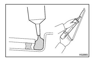
12. APPLY ADHESIVE TO MOULDING INSTALLATION AREA
