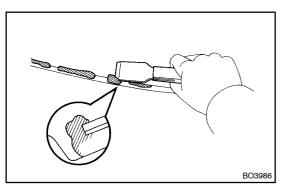
(c) Use a scraper to remove any excess or protruding adhesive.
