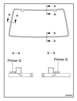
7. COAT CONTACT SURFACE OF BODY WITH PRIMER "M"
