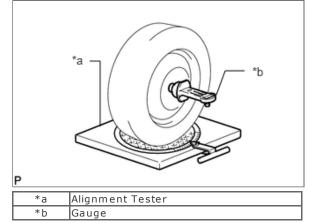
Install a camber-caster-kingpin gauge or place the front wheels on the center of a wheel alignment tester.
