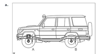
Press down on the vehicle several times to stabilize the suspension, and then measure the vehicle height.
