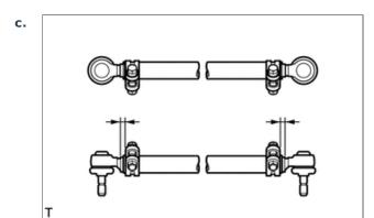
Make sure that the lengths of the left and right tie rod ends are the same.
