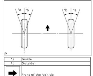
Turn the steering wheel fully, and measure the wheel angle.
