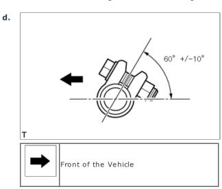
Tighten the clamp bolts and nuts.
