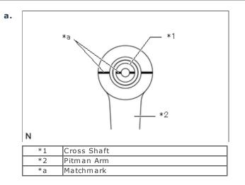
Align the matchmarks on the pitman arm and cross shaft.
