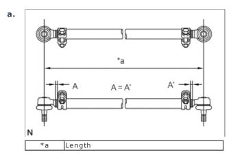
Turn the tie rod ends equal amounts into the steering tie rod, and adjust the length of the steering tie rod. Length:
