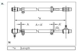
Turn the steering relay rod ends equal amounts into the steering relay rod, and adjust the length of the steering relay rod.
