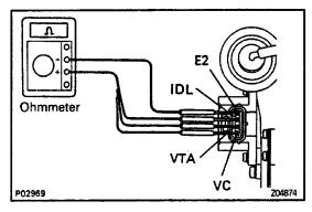
(d) Using an ohmmeter, measure the resistance between each terminal.
