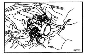
(b) Place a new gasket and install the throttle body with the 4 bolts.
