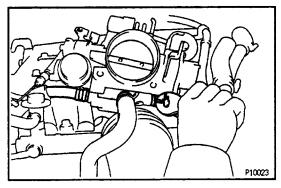
(b) Disconnect the No.4 and No.5 water bypass hoses from the throttle body.
