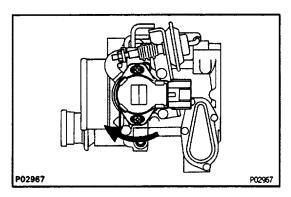
(d) Gradually turn the sensor clockwise until the ohmmeter deflects, and secure the sensor with the 2 screws.
