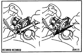
(e) If not as specified, adjust with the DP adjusting screw.
