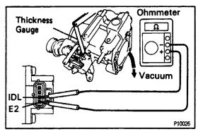
(e) Using a thickness gauge, recheck the continuity between terminals IDL and E2.
