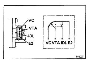
(c) Using an ohmmeter, measure the resistance between each terminal.
