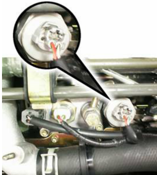
Ill.2 Alternative pump connection
